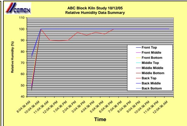
Figure 3 (Relative Humidity Analysis of Kiln)
