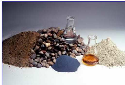
The use of presoaked aggregates, admixtures and/or supplementary cementitious materials are common practices
