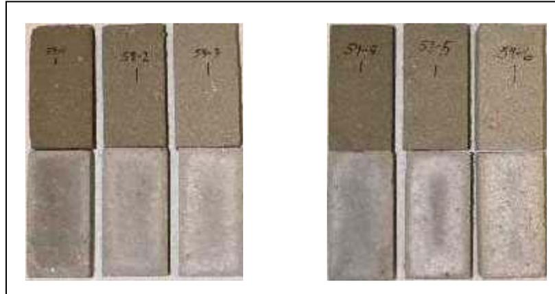
Figure 4 - Paver mixes with 13.6% (left set) and 18.3% (right set) cement
