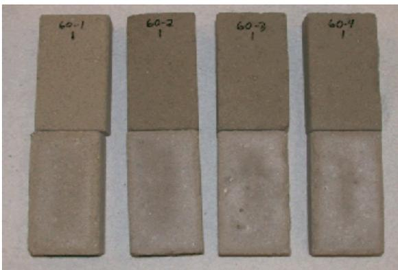
Figure 2 - Increasing cement contents (left to right)
