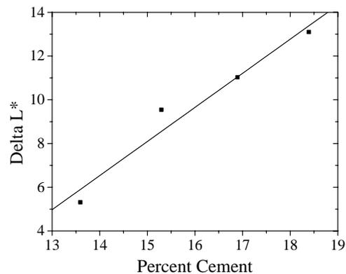
Figure 3 - Plotted change of  $L^*$  from 1 to 7 days
